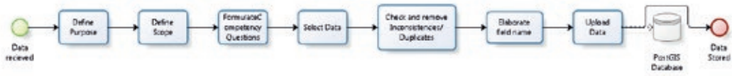
Figure 15 BPMN scheme of Phase 1 'prepare data' of the standardized workflow for publishing Linked Data
