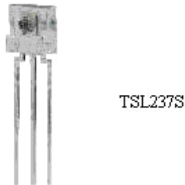
Figuur 7 TAOS TSL237S-lichtsensor, Bron: Texas Advanced Optoelectronic Solutions
