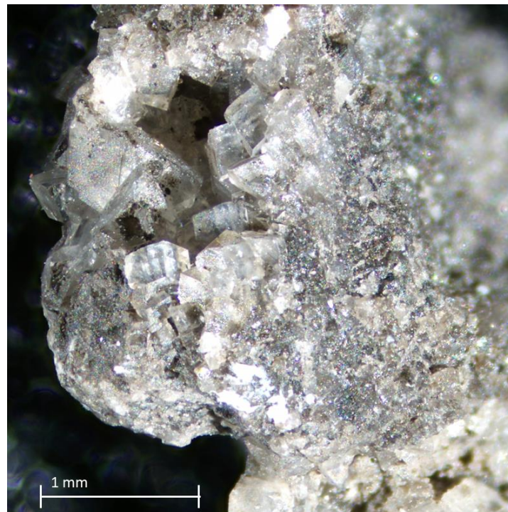
Figure 4: Euhedral calcite crystals developing around a cavity. Notice also the recrystallized nature of the grey colored limestone (“diagenesis reference sample” 1855m).
