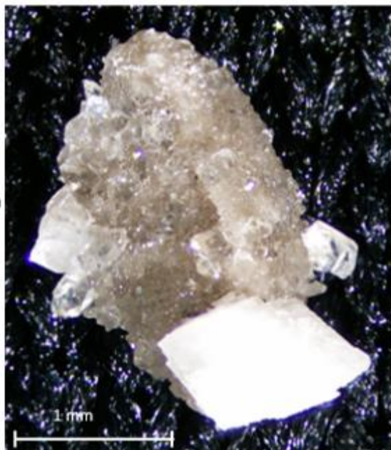
Figure 8: Calcite cement with well-developed crystals testifying of crystallization in open space ("diagenesis reference sample" 2120m).
