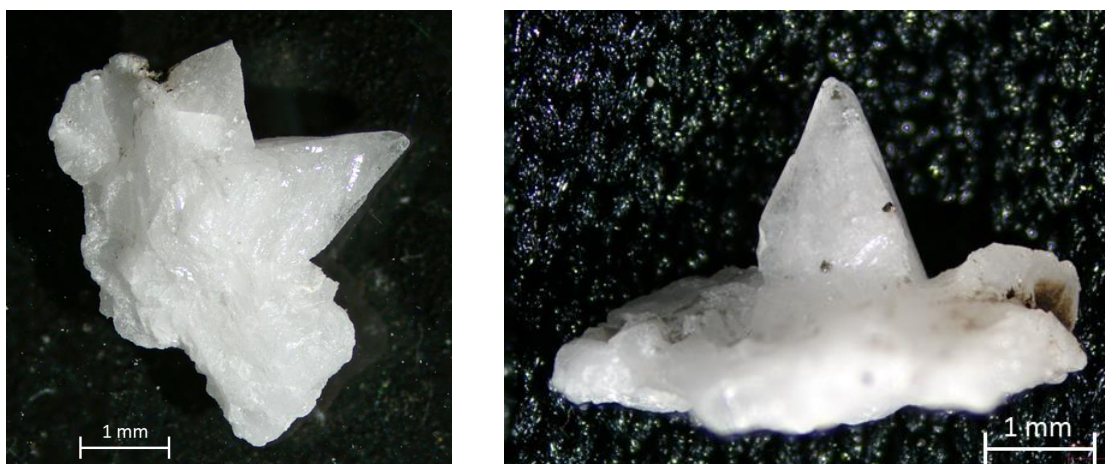
Figure 5: Calcite cement with well-developed skalenoides with minute pyrite crystals (right picture).-From the “diagenesis reference sample” set, 1950m.
