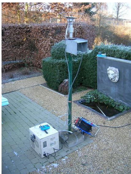
Figure 1 Equipment installed on each of the measuring locations: PDMS-Tenax sampler (PAH sampling) and Harvard impactor ( PM_{2.5} ) respectively mounted in and on the gray housing, which was attached to a metal stand. Both samplers were connected via rota-sil tubing to the respective pumps placed on the floor (left side of the stand)
